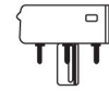
GX17q GX17q G17q DIN: 49665 IEC: 7004-45 ANSI: Four-pin prefocus base C81.61-1990 sheet I-440-1
